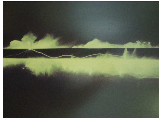
Figure 6. Propagating brush discharge from a plastic pipe conveying diesel fuel (photo courtesy J. F. Hughes, University of Southampton).
